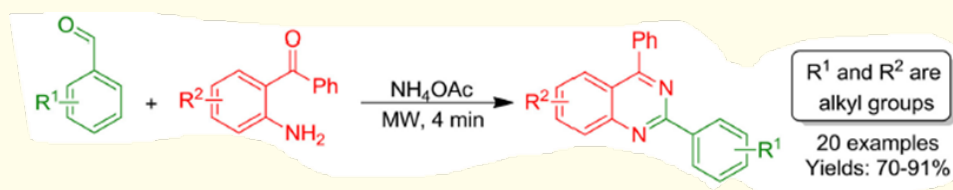
Scheme 5: Reaction of aldehydes and 2-aminobenzophenones under microwave heating conditions.
