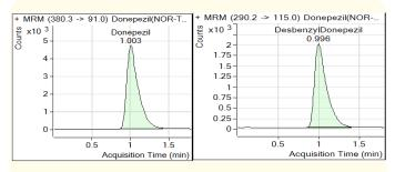
Figure 3: Chromatogram - an MRM data of blank plasma spiked with 20 ng/ml donepezil and internal standard desbenzyl donepezil.
