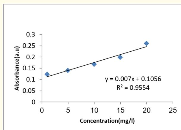
**Figure 5:** The linear calibration curve in the concentration range (1-20mg/l).
