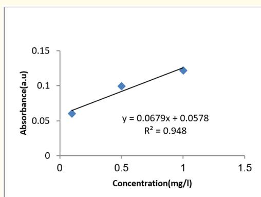
**Figure 4:** The linear calibration curve in the concentration range (0.1-1 mg/l).
