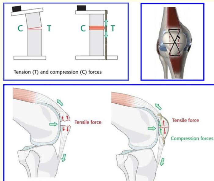
Figure 2: Principle of patellar tension band wiring.
