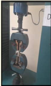
Figure 6: Breaking strength testing of shredded plastic mixture.
