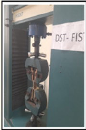
Figure 4: Study of breaking strength of potato starch solution mixed with Grinded plastic.
