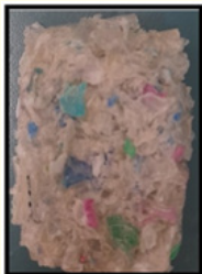
Figure 2: Shredded plastic waste mixed with potato starch solution.
