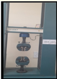
Figure 3: Study of breaking strength of the samples using the Universal Testing Machine.
