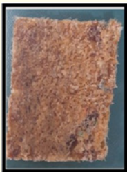
Figure 1: Grinded plastic waste mixed with potato starch solution.
