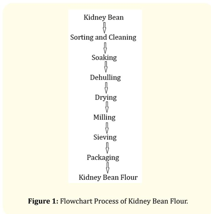
Figure 1: Flowchart Process of Kidney Bean Flour.
