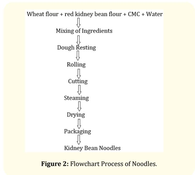
Figure 2: Flowchart Process of Noodles.
