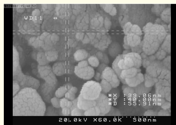
Figure 3: FESEM image of silver NPs.
