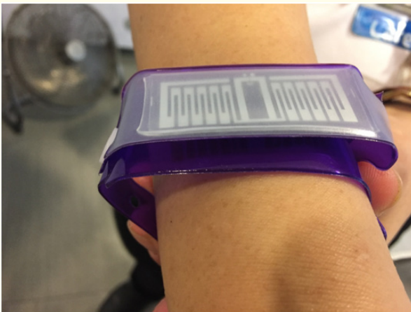
Figure 6: Security chip embedded in a wrist tag.
