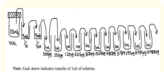
**Figure 2:** Illustration for the serial dilution procedure used for brands 'C', 'D', 'E', 'F', 'G', 'H', 'I', 'J' and 'K'.
