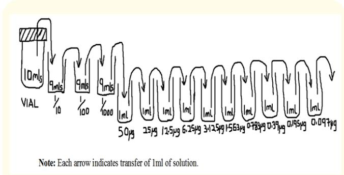
**Figure 1:** Illustration for the serial dilution procedure used for brands 'A' and 'B'.
