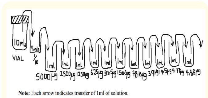
**Figure 3:** Illustration for the serial dilution procedure used for brands 'J' and 'H'.
