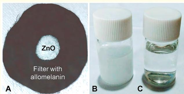
**Figure 2:** A: Allomelanin-impregnated fabric after filtering of the ZnO solution. Observe the white deposit of ZnO retained on the filter. B, C: Comparison between the aspect of 5 mL of milky ZnO solution before filtering (B), and clear solution filtered through the allomelanin-treated fabric (C).
