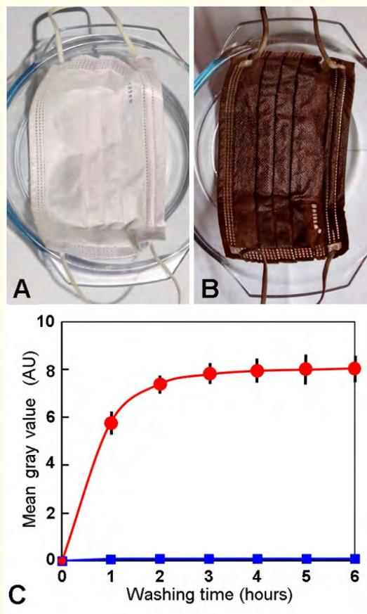
**Figure 1:** A, B: Commercial chin straps before (A), and after impregnation with allomelanin (B). C: Kinetics of the color removal of allomelanin-impregnated fabrics by water washing. The light brown color of 30 mL of washing media at increasing times (mean gray values in arbitrary units (AU), and standard deviation when pertinent) were measured by densitometry of photographs using ImageJ 1.52v software.
