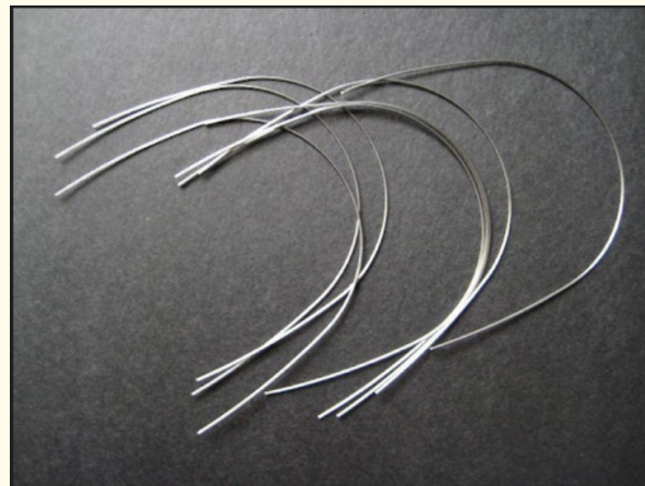
Figure 2: Nitinol arch wire which has shape memory.
