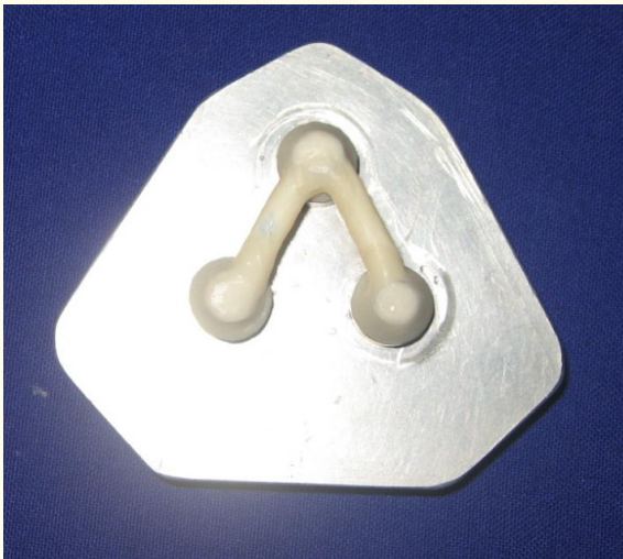
Figure 9: Pressed ceramic specimen.
