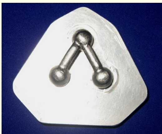
Figure 10: cp Titanium casting.
