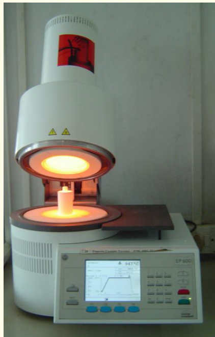
Figure 7: Furnace used for pressing ceramic.
