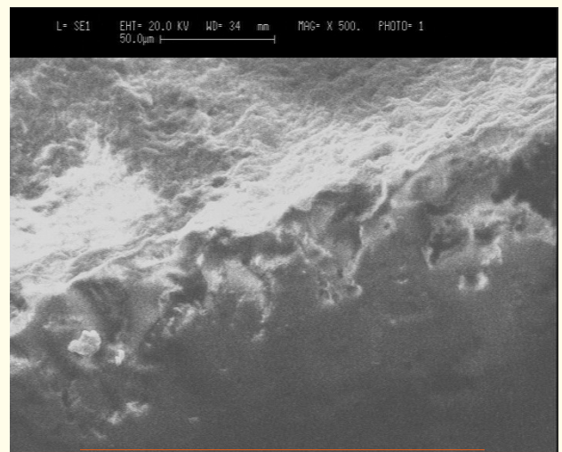
Figure 27: Adhesive failure through the interface of ceramic and composite resin.
