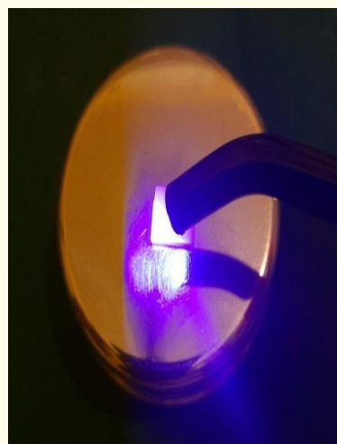
Figure 4: Light curing of NANOCOAT surface sealant.
