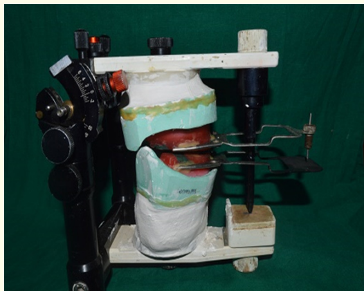
Figure 3: Tracer assembly seen, as mounted on a semi adjustable articulator. (In picture- Artex Semi adjustable (non arcon) Articulator, with Height tracer units attached).
