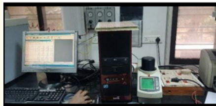
Figure 11: Testing of color stability using spectrophotometer.
