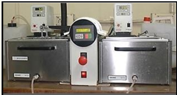
Figure 9: Thermocycling of Test Samples.
