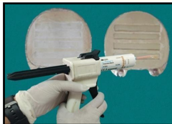
Figure 5: Fabrication of the BIS- ACRYL samples. Fabrication of group C specimens (visible light cure resin).
