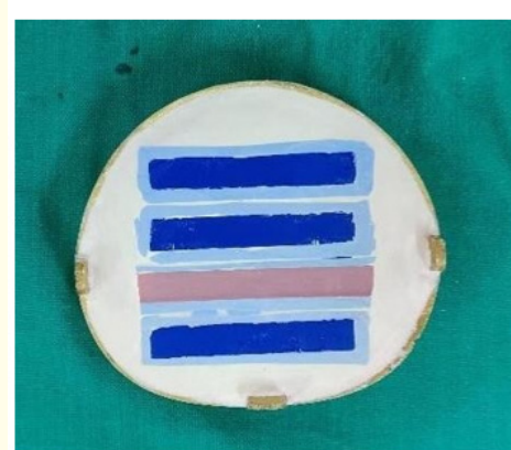
Figure 2: Milled Wax bar specimens invested in brass varsity flask.
