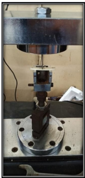
Figure 10: Testing of flexural strength using universal testing machine.
