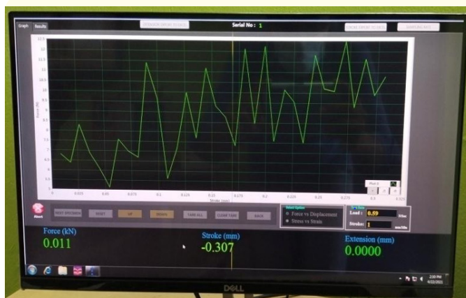
Figure 5: Recording of maximum load at fracture (3D printed resin).
