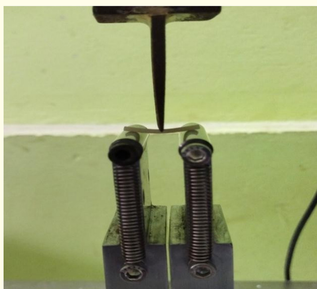
Figure 4: Application of load at the center of the sample (3D printed resin).
