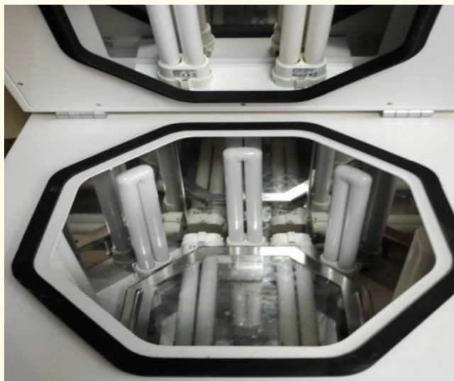
Figure 3: Group II samples in NEXTDENT 5100 post curing unit.
