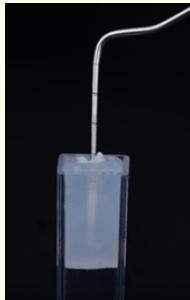
Figure 3: Packing of composite inside the transparent mold.
