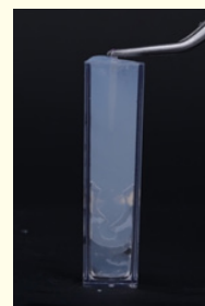
Figure 1: Fiber post inserted into the soft impression material.
