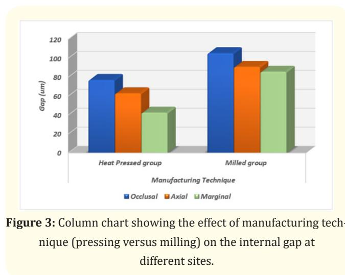
**Figure 3:** Column chart showing the effect of manufacturing technique (pressing versus milling) on the internal gap at different sites.
