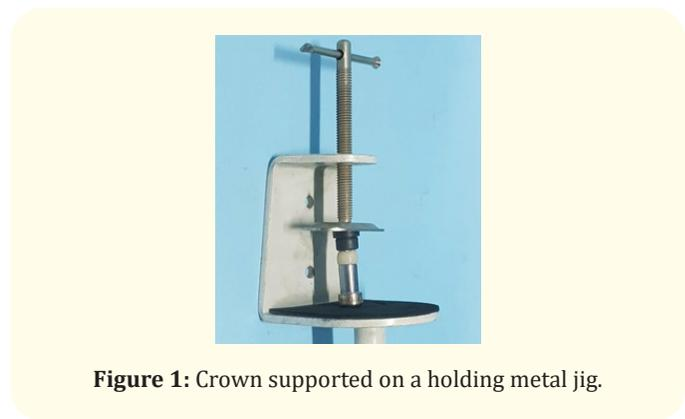
Figure 1: Crown supported on a holding metal jig.
