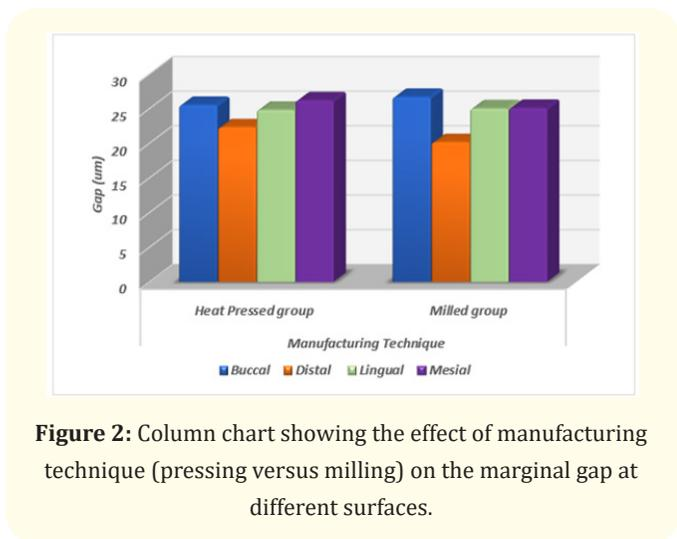
**Figure 2:** Column chart showing the effect of manufacturing technique (pressing versus milling) on the marginal gap at different surfaces.
