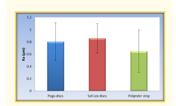
Figure 7: Bar chart representing mean and standard deviation values for Ra of different polishing systems regardless of other variables.
