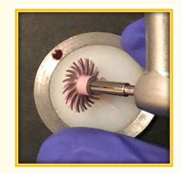
Figure 5: Polishing the specimen with the Sof-Lex ultra fine (Pink).
