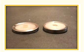
**Figure 1:** The specimens were inserted into the second Teflon mold, marked on the side to facilitate the polishing procedures.
