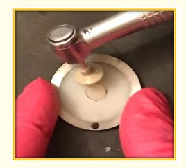
Figure 2: Polishing the specimen with PoGo micro-polisher disc.
