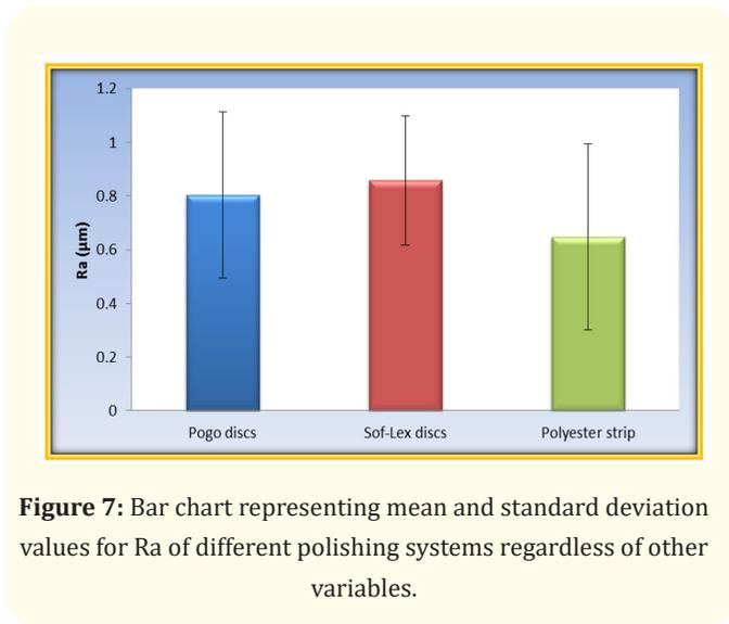
**Figure 7:** Bar chart representing mean and standard deviation values for Ra of different polishing systems regardless of other variables.
