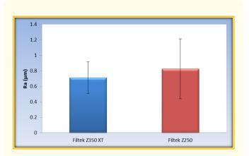
Figure 6: Bar chart representing mean and standard deviation values for Ra of the two composite types regardless of other variables.
