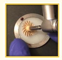
Figure 4: Pre-polishing the specimen with the Sof-Lex spiral wheel fine (beige).
