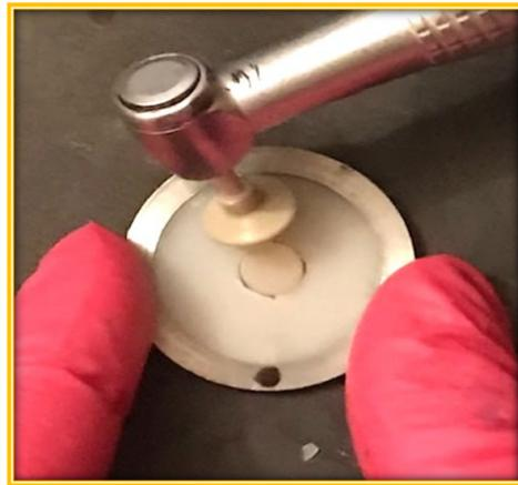
**Figure 2:** Polishing the specimen with PoGo micro-polisher disc.
