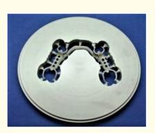
**Figure 9:** CAD CAM milled RPD framework. (Source: https://www.dentalcadcamshop.com/production/blocks-forcerec-inlab/ernst-hinrichs/juvora-dental-peek.html.)
