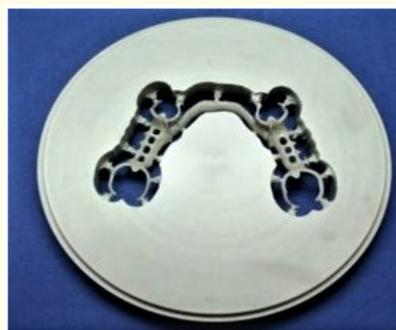
**Figure 9:** CAD CAM milled RPD framework.
