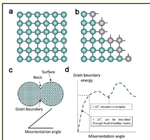
**Figure 3:** a) A single crystal structure in which the atoms are arranged in a repeating pattern and the atomic bonds are connected between them; b) A single crystal free surface with a disrupted atomic bond. Surface energy is induced by dangling atomic bonds; c) a schematic of two disoriented nanoparticles with an illustration of the disorientation angle; and d) grain boundary energy charges with a disoriented angle [12].
