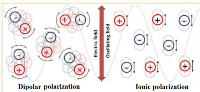
**Figure 1:** Diagram of dipolar polarization (dipoles align in the microwave field) and ionic conduction mechanisms of dielectric heating (ions move in the microwave field) [4].
