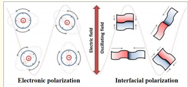
**Figure 2:** The electronic polarization mechanism (movement of charges in the microwave field) and the interfacial mechanism are shown schematically in this dielectric heating diagram (accumulation of charges on the interface between two different surfaces) [4].
