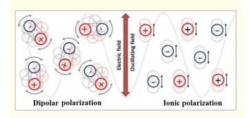
**Figure 1:** Diagram of dipolar polarization (dipoles align in the microwave field) and ionic conduction mechanisms of dielectric heating (ions move in the microwave field) [4].
