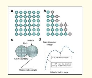
Figure 3: a) A single crystal structure in which the atoms are arranged in a repeating pattern and the atomic bonds are connected between them; b) A single crystal free surf ace with a disrupted atomic bond. Surface energy is induced by dangling atomic bonds; c) a schematic of two disoriented nanoparticles with an illustration of the disorientation angle; and d) grain boundary energy charges with a disoriented angle [12].
