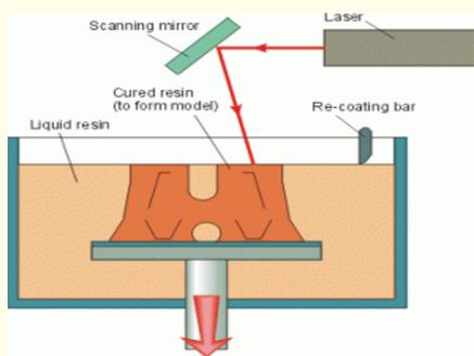
**Figure 2:** Stereolithography printing (adapted from 3D-printing expert.com)
