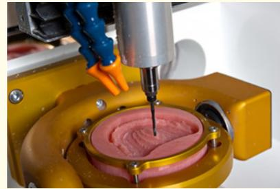
**Figure 1:** Milling of dentures: AvaDent denture being milled from a Lucitone 199@puck. ([https://lmtmag.com/articles/technology\\_to\\_watch\\_avadenttrade\\_digital\\_dentures/photos](https://lmtmag.com/articles/technology_to_watch_avadenttrade_digital_dentures/photos))
