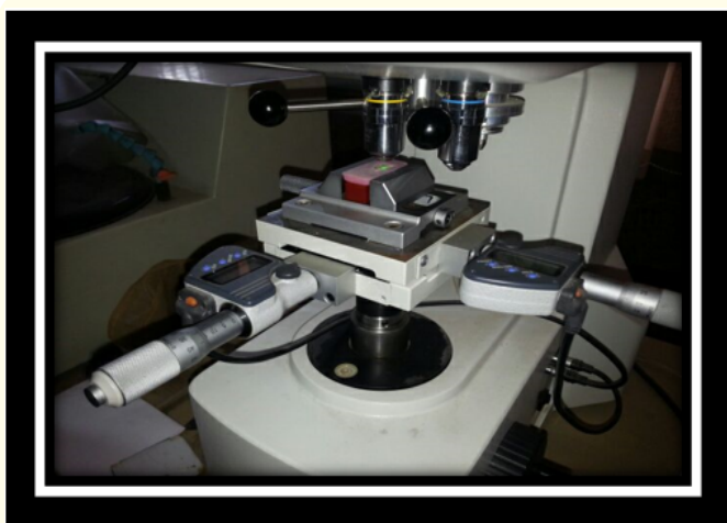
Figure 3: Specimen mounted on Vickers.
