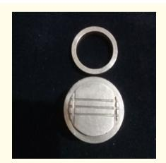
Figure 2: Standardized metal die as per ADA specification number #19.
