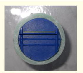
**Figure 4:** Measuring the distance from the inner profile of the two cross vertical lines of impressions.
