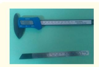
Figure 1: Digital Vernier Caliper.
