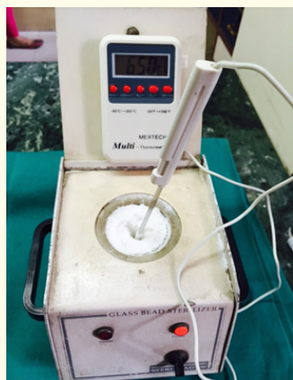
Figure 1: Glass Bead Sterilizer with common salt and digital thermometer placed to verify temperature.
