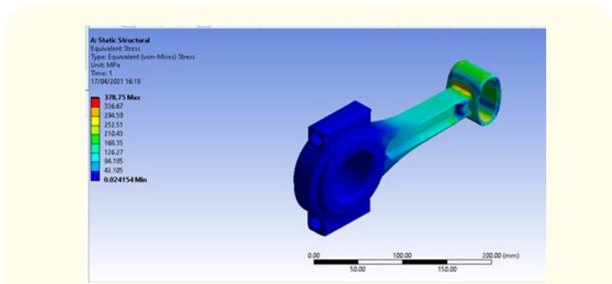
Figure 9: Equivalent (Von Mises) Stress of Structural Steel Material.
