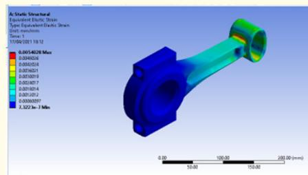
Figure 16: Equivalent Elastic Strain of Aluminium 7075 T6 Alloy.
