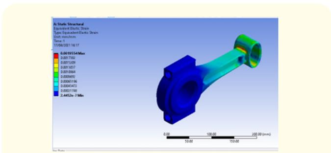
Figure 8: Equivalent Elast Strain of Structural Steel Material.
