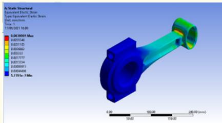
Figure 4: Equivalent Elastic Strain of Titanium Alloy Material.
