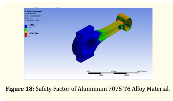
Figure 18: Safety Factor of Aluminium 7075 T6 Alloy Material.
