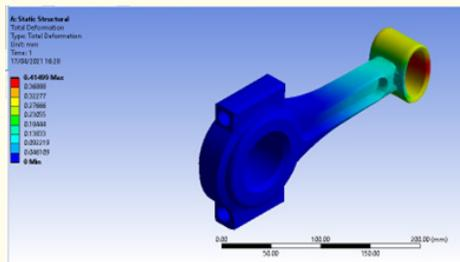
**Figure 11:** Total Deformation of Gray Cast Iron Material.
