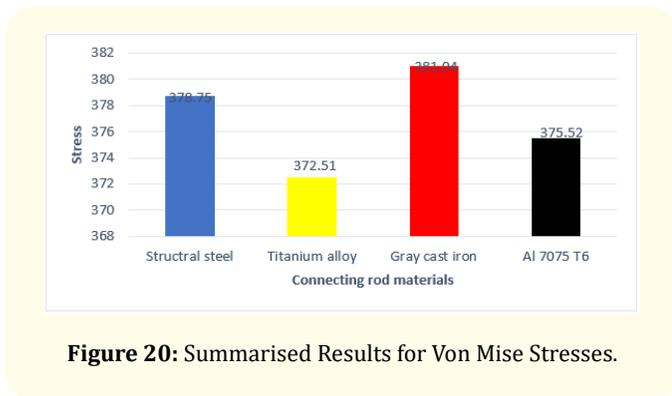
Figure 20: Summarised Results for Von Mises Stresses.
