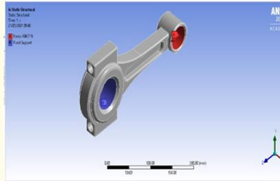
Figure 2: The boundary condition for the analysis.
