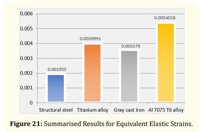
Figure 21: Summarised Results for Equivalent Elastic Strains.
