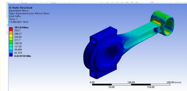
**Figure 13:** Equivalent (Von Mises) Stress of Gray Cast Iron Material.
