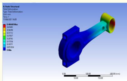
Figure 3: Total Deformation of Titanium Alloy Material.
