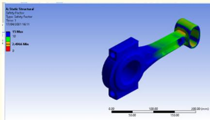
Figure 6: Factor of Safety of Titanium Alloy Material.
