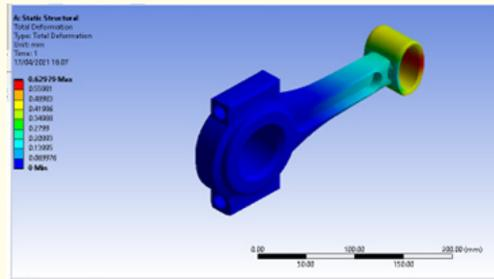
Figure 15: Total Deformation of Aluminium 7075 T6 Alloy.
