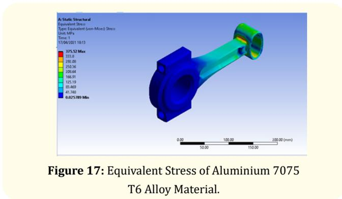
Figure 17: Equivalent Stress of Aluminium 7075 T6 Alloy Material.
