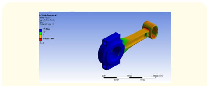
Figure 10: Safety Factor of Structural Steel Material.
