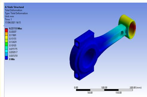
Figure 7: Total Deformation of Structural Steel Material.
