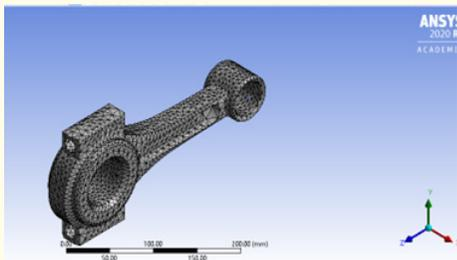
Figure 1: Connecting rod Meshed in Ansys.
