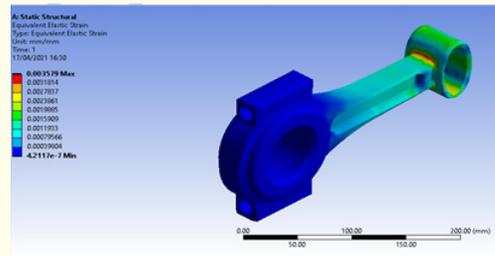
**Figure 12:** Equivalent Elastic Strain of Gray Cast Iron material.
