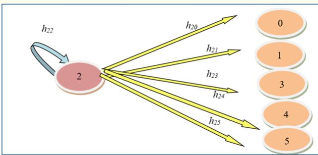
**Figure 2:** A schematic diagram which shows the elements of traffic pattern matrix corresponding to a packet generated at node 2 and directed to the 6 nodes in  $K=6$  topology
