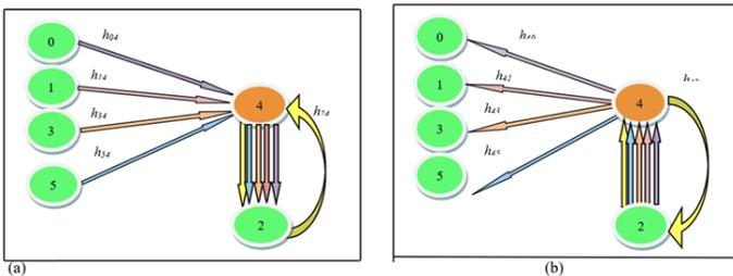
**Figure 3:** A 6-node Bluetooth piconet where node 4 is the master and node 2 is under observation (a) Traffic to node 2 (b) Traffic from node 2.
