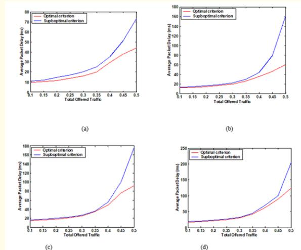
**Figure 4:** Variation of the average packet delay obtained by using the optimal criterion and suboptimal criterion with total offered traffic for (a) 5-node piconet (b) 6-node piconet (c)7-node piconet (d) 8-node piconet.
