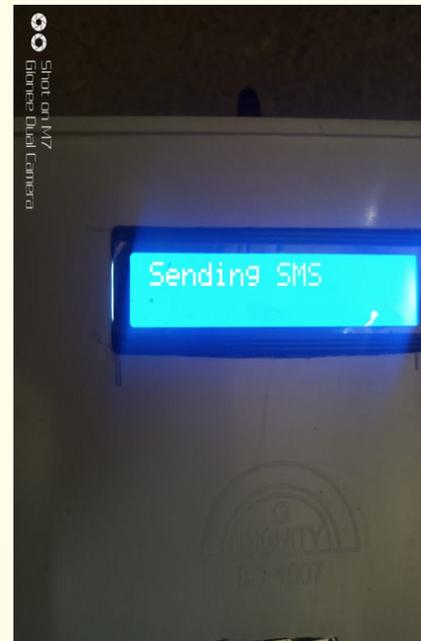
**Figure 7:** Sending SMS from the implemented system to the registered phone number.
