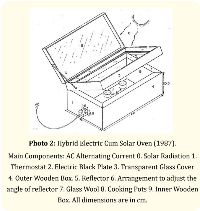
**Photo 2:** Hybrid Electric Cum Solar Oven (1987).
