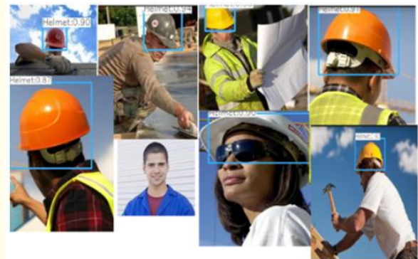
Figure 2: Checking the worn helmet on the construction site by image analyzing [19].
