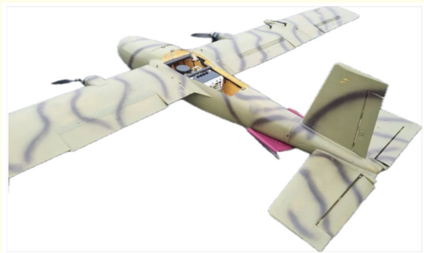
Figure 1: UAV model "Os'-25" equipped with the airborne "TOR" device.
