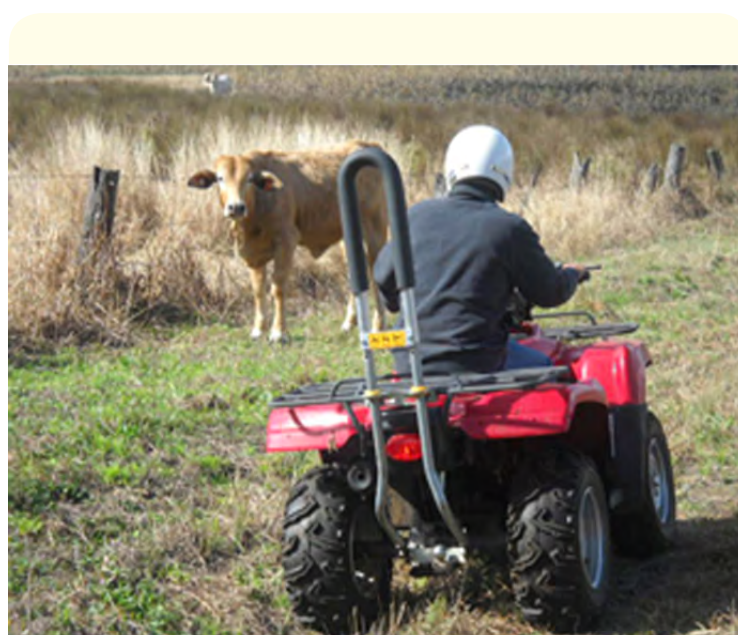
Figure 1: Quadbar™ fitted onto an ATV.
