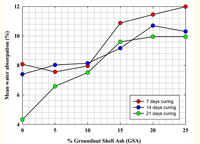
**Figure 6:** Mean water absorption of the cement block as a function of groundnut shell ash.
