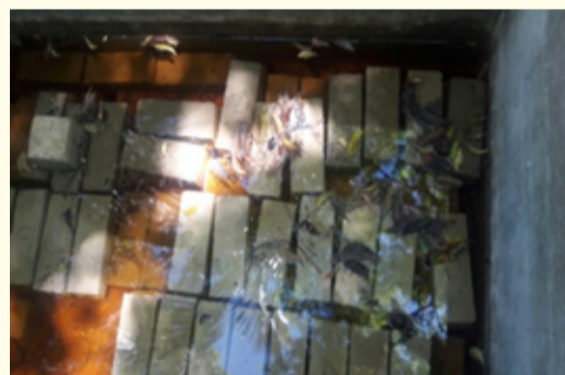
Figure 3: GSA-Cement blocks were immersed into the water for one day in the temperature range of 25 to 30°C.
