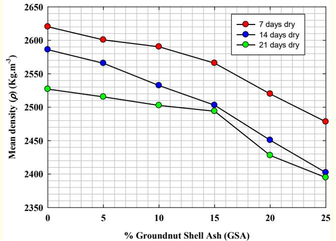
**Figure 5:** Mean density of the cement block as a function of groundnut shell ash.
