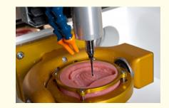
**Figure 1:** Milling of dentures: AvaDent denture being milled from a Lucitone 199®puck. (https://lmtmag.com/articles/technology\_to\_watch\_avadenttrade\_digital\_dentures/photos)
