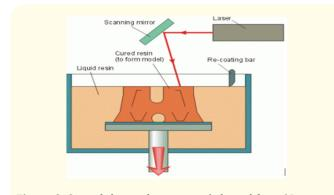
Figure 2: Stereolithography printing (adapted from 3D-printing expert.com)
