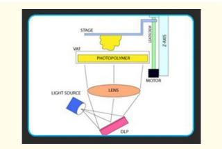
Figure 3: Digital light processing printing method (adapted from 3D-printing expert.com)
